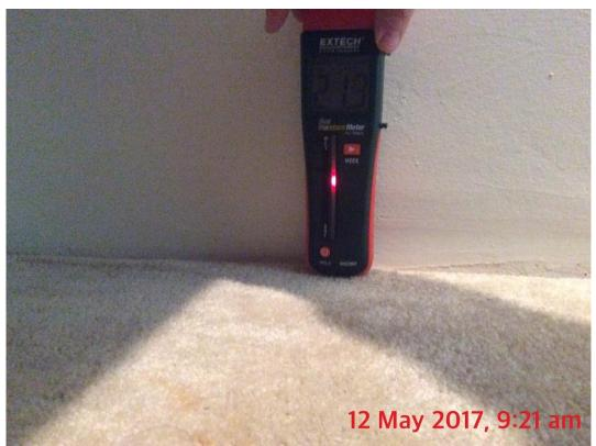
Picture No.1 showing moisture reading between Bathroom and Linen – 21.3
