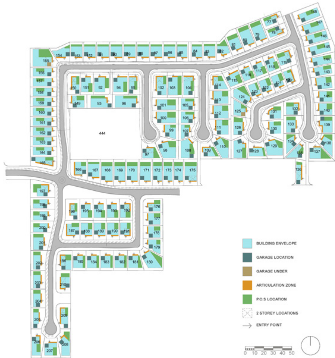
Figure 2 Site analysis/building envelopes
