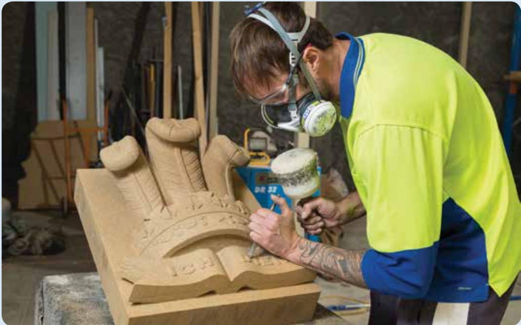
The Prince's Feathers, carved by a local stone mason in locally sourced stone, will adorn the front of the Terrace.
